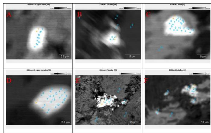
Fig 4. Exemplary BSE microphotographs of the new phases: A. Telluroplatinumpalladinite (Phase 3); B. bright center are Pb-Kotulskite (phase 2b), point -7 Pb-mitrofanovite (phase 2a); C. Platinumtörnroosite (phase 6b); D. Ag-Telluropalladinite (phase 1b); E. Ag-Maslovite (phase 1); F. bright center are Ag-Kotulskite (phase 1a).
